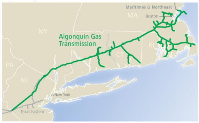
The Algonquin Gas Transmission pipelines transport 2.6 Bcf/d through 1,127 miles of pipeline. Algonquin connects to Texas Eastern Transmission and Maritimes & Northeast. Its peak day design capacity enables us to offer abundant and reliable natural gas at competitive rate
