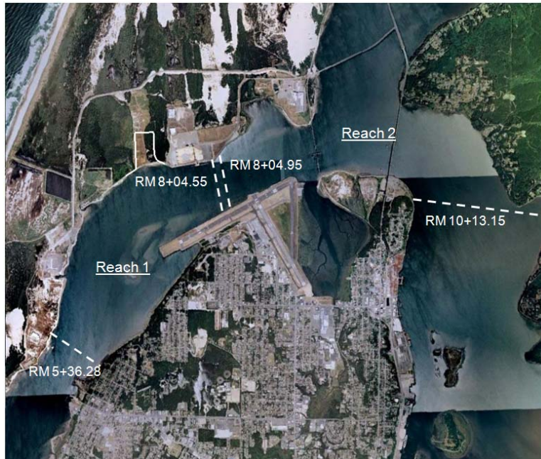
Figure 3. Federal Navigation Channel reaches with maintenance dredging over last 20 years
