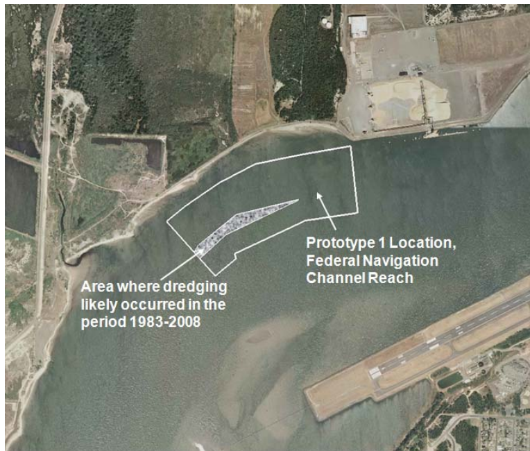
Figure 6. Area of previous dredging work according to USACE
