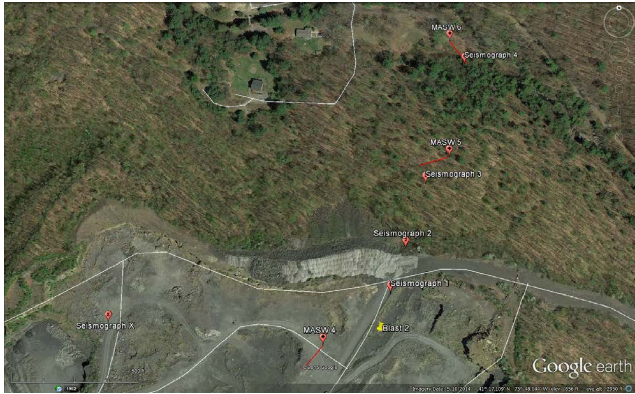
Figure 4 - Locations of MASW Surveys Near Blast 2 Seismographic Array
