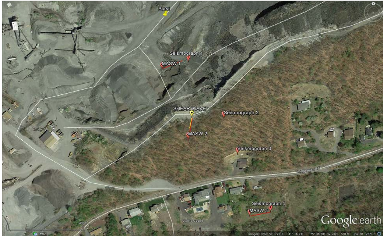
Figure 3 - Locations of MASW and Apparent Shear-Wave Velocity Surveys Near Blast 1 Seismographic Array
